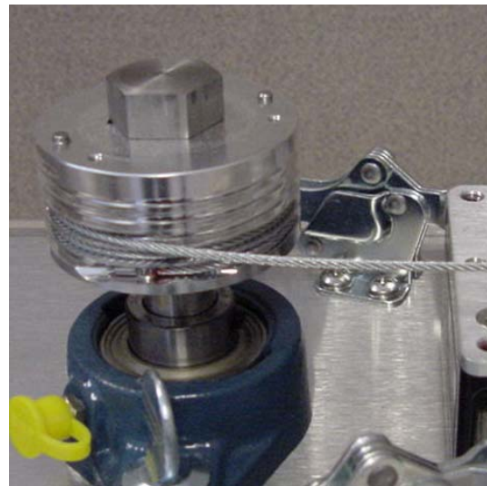
Figure 3-7. Cable Placement (fixture capstan)
