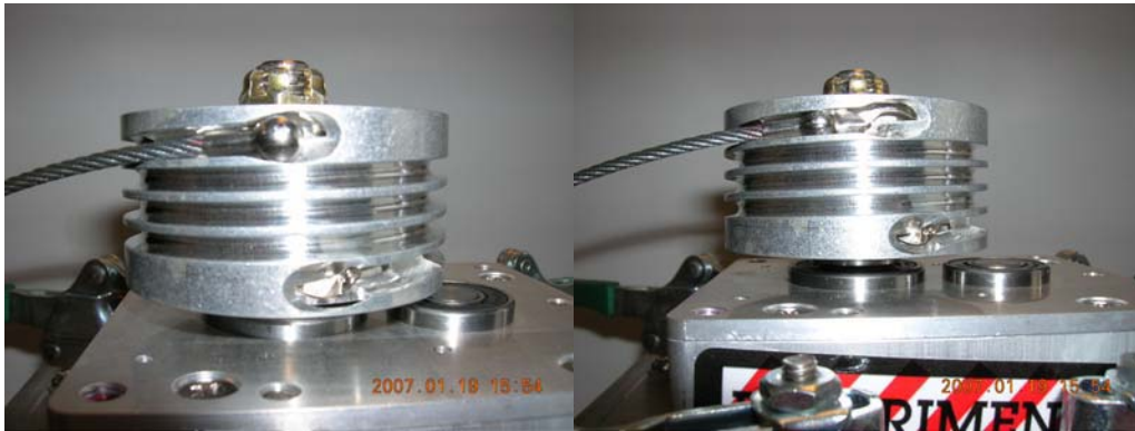
Figure 3-10. Inserting 3/32 cable in the unit capstan.
