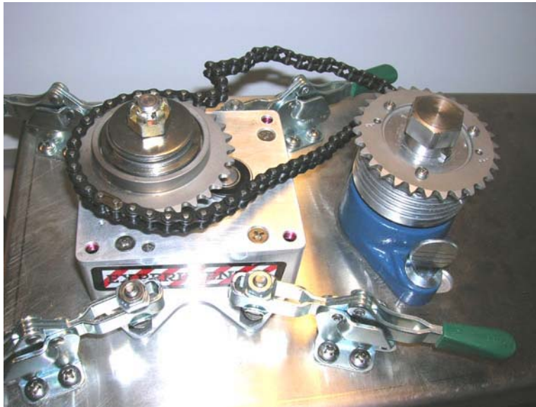
Figure 3-24. Sprocket capstan installed on fixture
