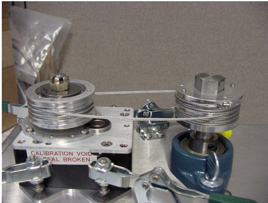
Figure 3-9. Cable End Placement (unit capstan)
