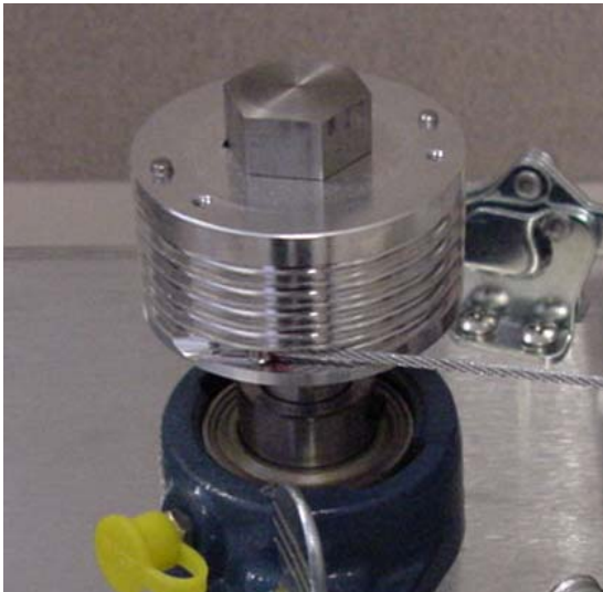
Figure 3-6. Cable Placement (fixture capstan)
