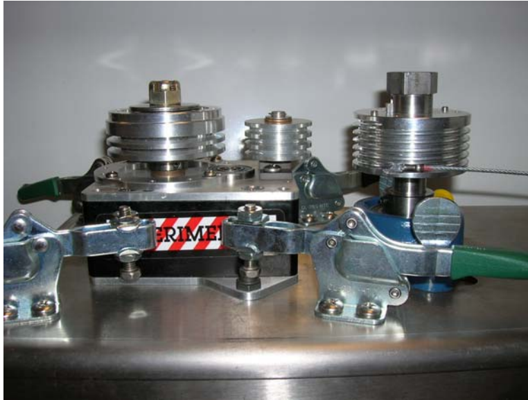
Figure 3-16. Cable end inserted in bottom slot
