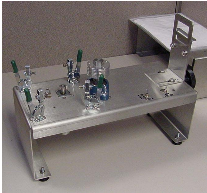
Figure 3-3. Slip-Clutch Adjustment Fixture (P/N T10-00110-01)
